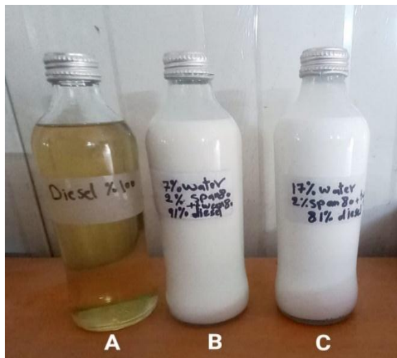
Figure 1. Fuel types used in the present study: (A) Pure diesel, (B) water diesel emulsion 7%, (C) water diesel emulsion 17%.
